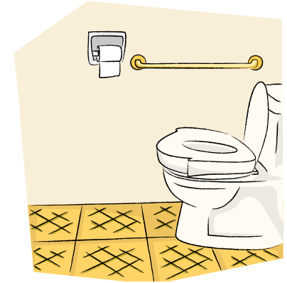
After: A sitting toilet with an additional toilet raiser, installation of grab bar and anti-slip floor treatment.
