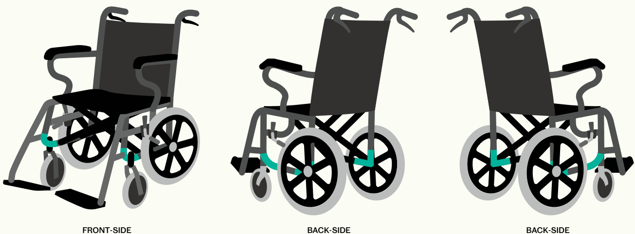
Fig 34: Wheelchair with appropriate securement points marked out with coloured and contrasting tape
